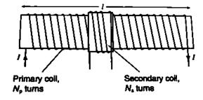
26- If the current in the primary coil decreases uniformly from 12.0 A to zero in 58.0 ms and the  $(\Delta V_{ind})$  induced in the secondary coil is 8.03 V, calculate the mutual inductance, M.
