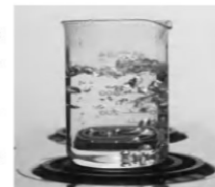
Figure 5 As temperature increases, the particles that make up a substance in its liquid state move faster. When their energy creates sufficient pressure to surpass the air pressure above the liquid, the liquid boils.
