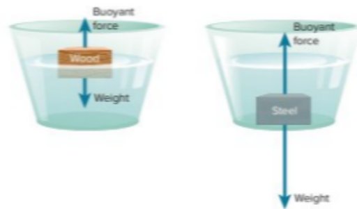
Figure 13 The steel block sinks because the buoyant force from the fluid is less than the gravitational force on the object. When the buoyant force is the same as or greater than the gravitational force—as with the wooden block—the object floats.
